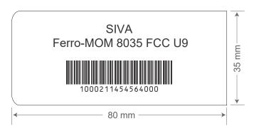
SIVA's Ferro-MOM 8035 FCC U9 is a passive RAIN (UHF) RFID label optimized for Metal surfaces and delivered with a high performance permanent adhesive with excellent bonding. These labels feature a film face to print customized logos, product information, scannable barcodes, QR codes, etc. directly on the label.
