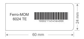
SIVA's Ferro-MOM 6024 TE is a non-transferable tamper-evident label for Mount on Metal applications demanding long read range in small form factor with a high performance permanent adhesive. Supplied in roll form as finished label and it can be encoded and printed with typical RFID printers that are capable of printing labels.
